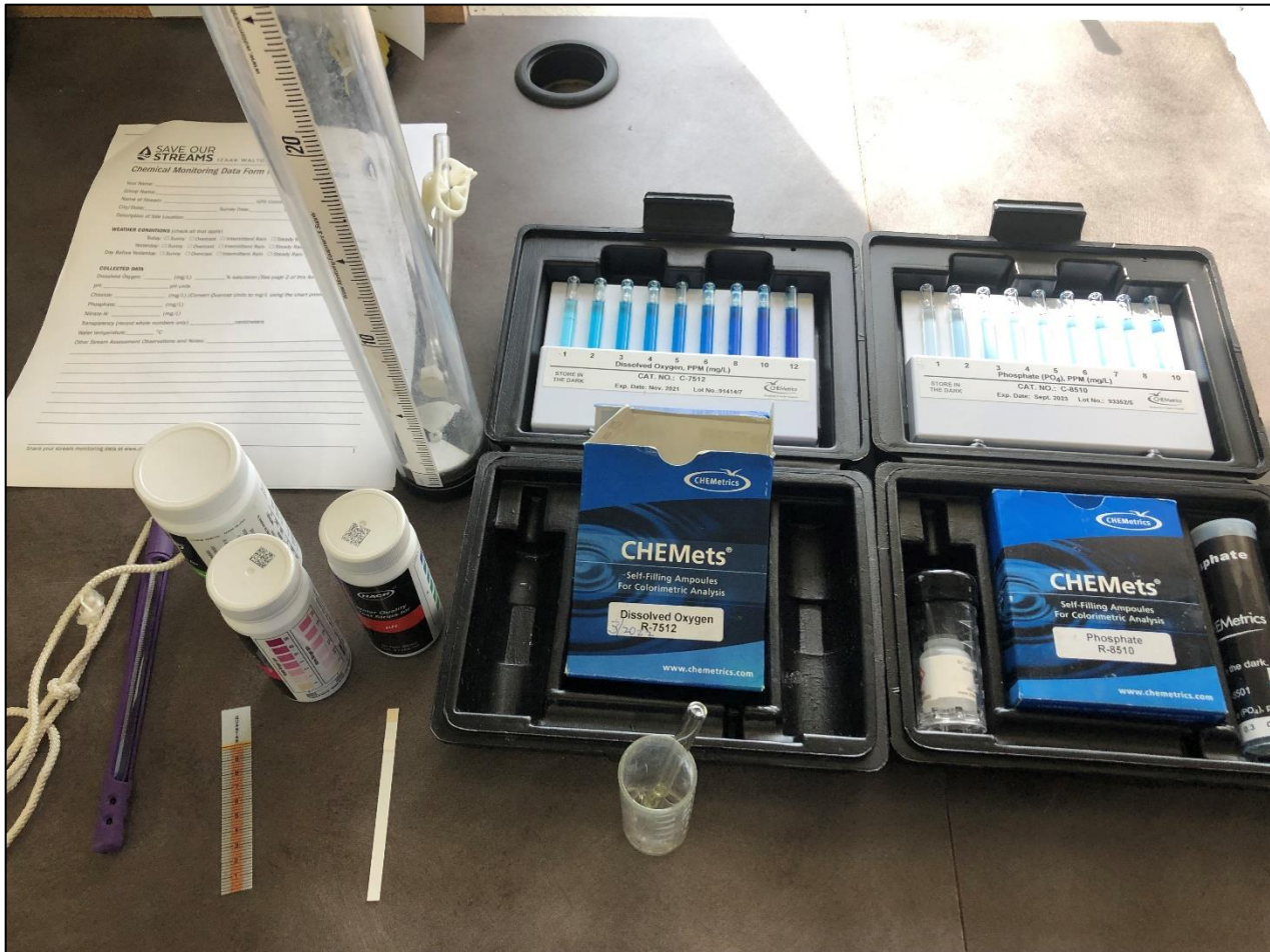
An example of a kit for monitoring water chemistry. Nitrate, pH, and chloride are measured with Hach test strips, orthophosphate and dissolved oxygen with Chemetrics ampoules, water clarity is measured with a transparency tube, and water temperature is measured with a thermometer.
