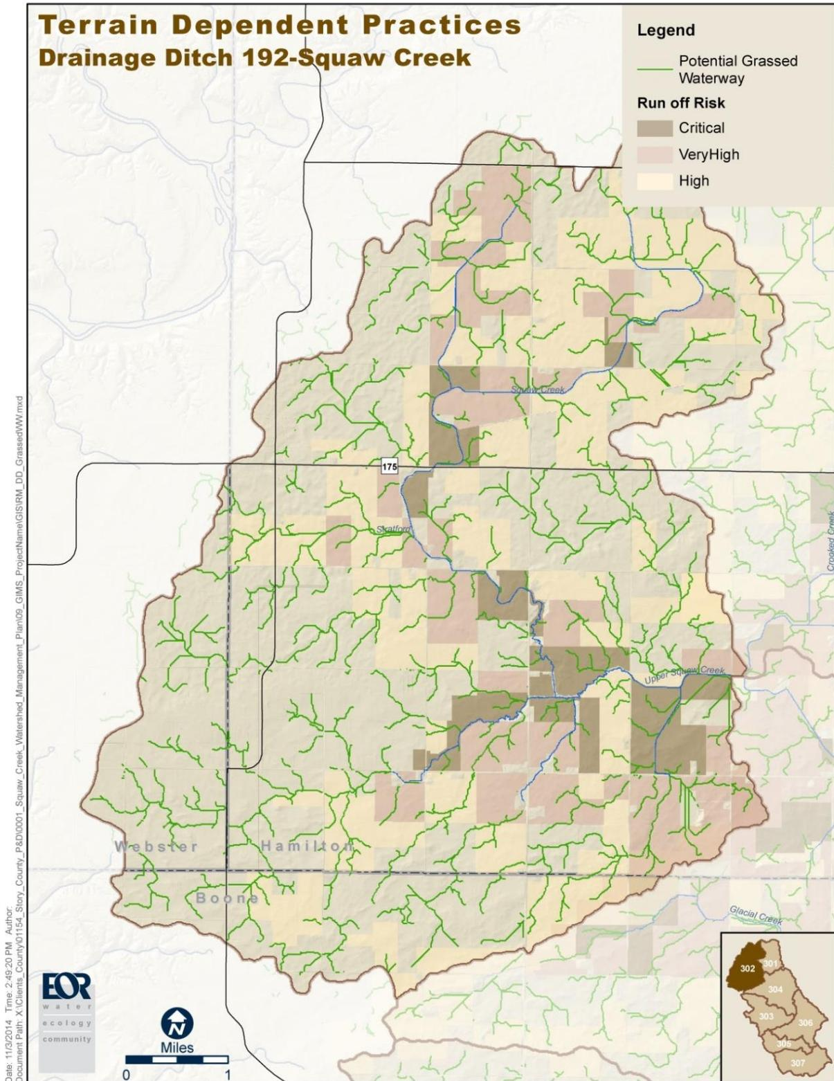
**A4 Figure 5.** Potential grassed waterway sites and soil runoff risk in Drainage Ditch 192 – loway Creek Subwatershed.
