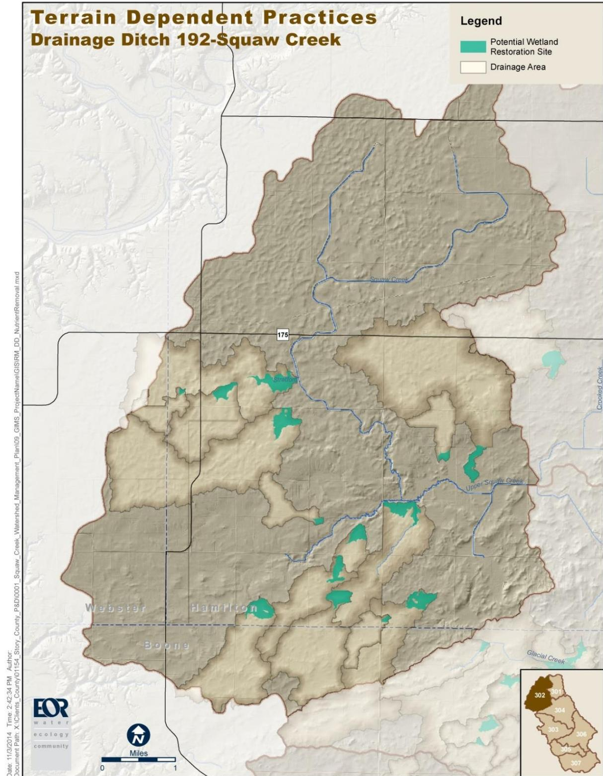
**A4 Figure 6.** Potential nutrient removal wetland sites in Drainage Ditch 192 – loway Creek Subwatershed.
