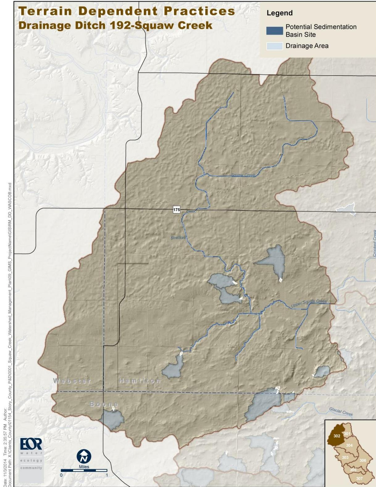
**A4 Figure 7.** Potential sediment basin sites in Drainage Ditch 192 – loway Creek Subwatershed.
