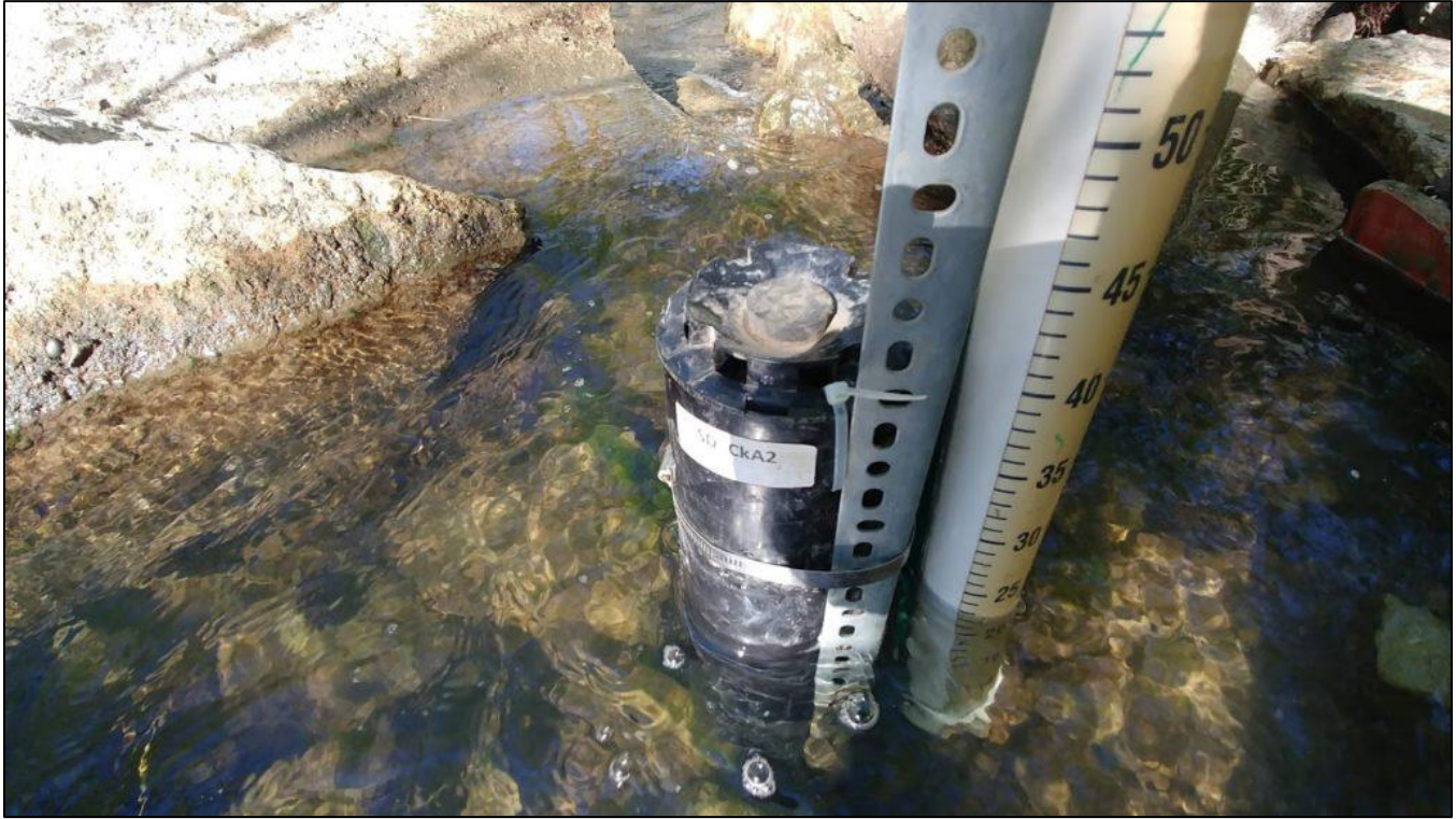
Mounting hardware for a Nalgene storm sampler, installed in a stream. A crest-stage recorder measures the rise in water level.
