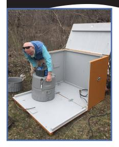
Prairie Rivers of Iowa, in collaboration with the City of Ames, installed an automatic monitoring station on Squaw Creek at Lincoln Way in Ames. The monitoring unit takes monthly grab samples and extra samples at times of high flow after rain events. The samples are collected from the monitoring unit and taken to be analyzed by the lab technicians at the state-certified lab in Ames.
